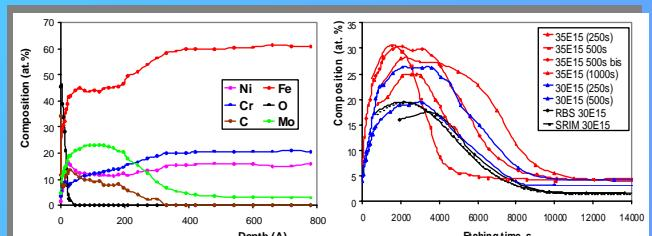
High carbon concentration is detected in the implanted layer
