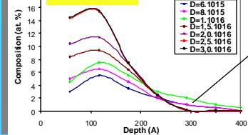
For high implantation current density, implanted layer is thicker
