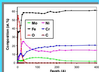
No carbon is detected in implanted layer
