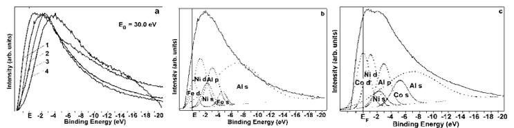
Electron spectra in valence band region of alloys on base of nickel aluminide: (a) 1 NiAl(Co) 2 NiAl(Fe); 3 NiAl; 4 NiAl(Mo); and interpretation of density-of-states in VB of alloyed intermetallic: (b) NiAl(Fe); (c) NiAl(Co). ( $E_0=30.0$  eV).
