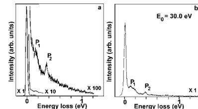
HREEL spectra of polycrystalline surfaces of NiAl (a) and NiAl(Fe) alloy (b). Primary beam energy 30 eV.
