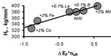
Correlation between micro-hardness and electronic structure characteristics of alloys on base of NiAl.
