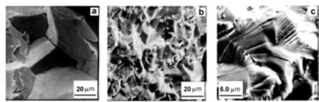
SEM images of inter-granular fracture of NiAl intermetallic (a), quasi-cleavage fracture of NiAl(Co) alloy (b) and dislocation slip transmission across grain boundaries in NiAl (La) alloy (c).
